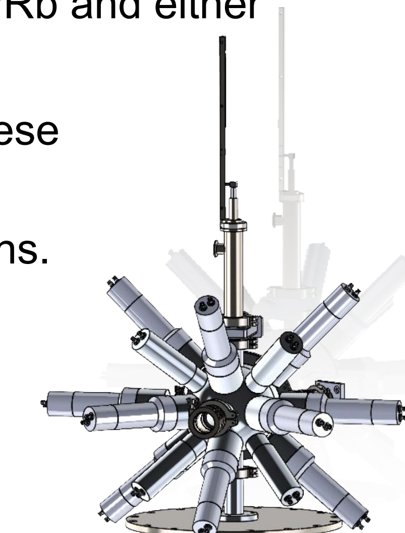
Figure 8: Planned CeBrA consisting of 14 CeBr 3 detectors.
