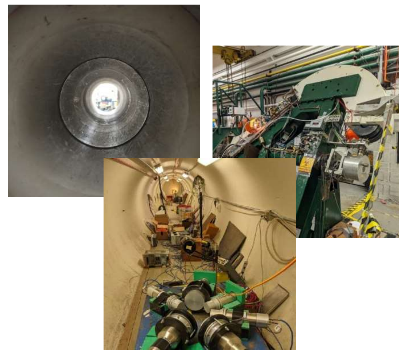
Fig. 1: CATRiNA neutron detector array in neutron tunnel at Edwards Accelerator Laboratory.
