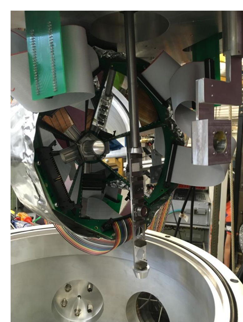
(top and from left to right) CeBrA demonstrator in front of SE-SPS, proton- \gamma coincidence matrix for ^{52}\text{Cr}(d,p)^{53}\text{Cr} , and proton- \gamma angular correlations for 3707-keV state in ^{53}\text{Cr} . (bottom and from left to right) Lampshade design of SABRE's silicon detectors, SABRE being mounted inside scattering chamber, and SABRE-SE-SPS coincidence matrix.
