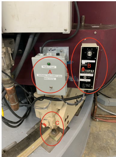
Figure 10: Magnet Motor controls A) Motor power B) Speed and direction control C) Angle readout
