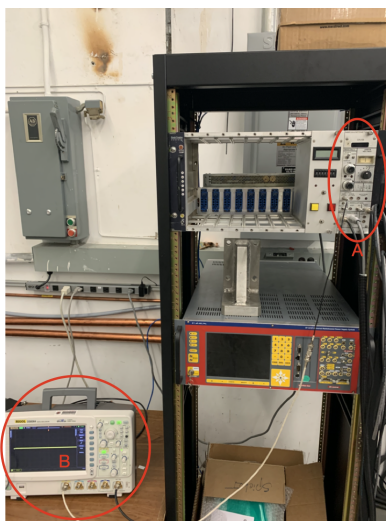
Figure 3: NMR Probe Readout and Settings A) Probe control and readout module B) Oscilloscope for viewing waveforms
